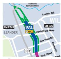
Extension will be a limited-access toll road with three lanes in each direction. It will be constructed in the median of the existing frontage roads, from RM 1431 to jut north of RM 2243. The frontage roads will remain non-tolled. Design work should be completed by this summer, and depending on financing, construction could be underway by the end of the year.
